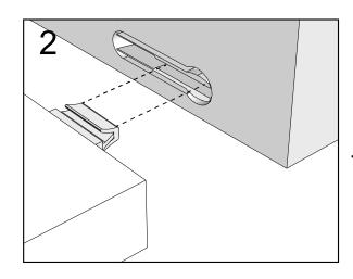
Push connector into housing to join.
