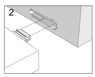
Push connector into housing to be jointed.
