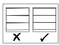
Please ensure all doors and drawers are aligned and evenly spaced before applying the back panel fixings.
