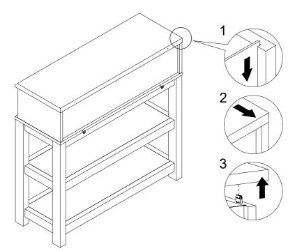
Press the back panels downward so that the top panel can be slide off.
