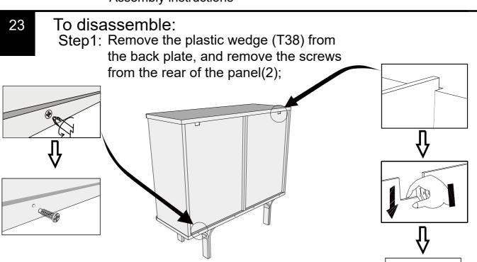
Step2: Press down the two back panels so they are clear of the top panel slot;
