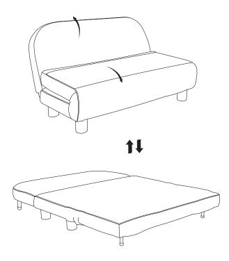
When transforming into the bed position, unzip & remove the foam pads from the seat to release the supporting legs. Then fold the seat down.
