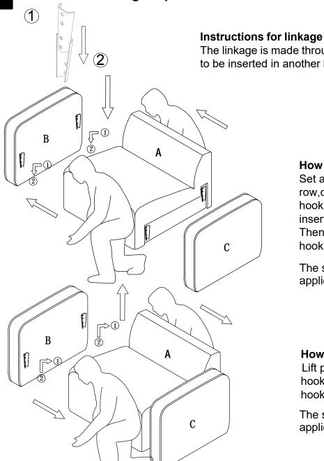
The linkage is made through a hook (1) to be inserted in another hook (2).
