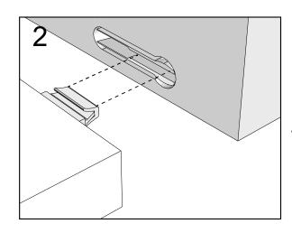
Push connector into housing to join.
