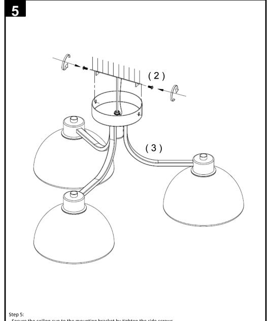
$\mbox{-}$  Secure the ceiling cup to the mounting bracket by tighten the side screws.
