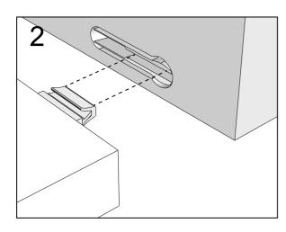
Push connector into housing to be jointed.
