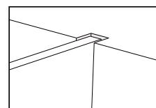
Step2: Press down the back panel so it is clear of the top panel slot;
