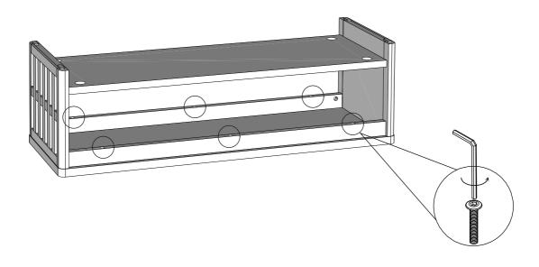
Slide the top panel front to unlock, then lift off. Follow the same sequence to remove the other panels;
