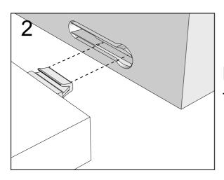
Push connector into housing to be jointed.
