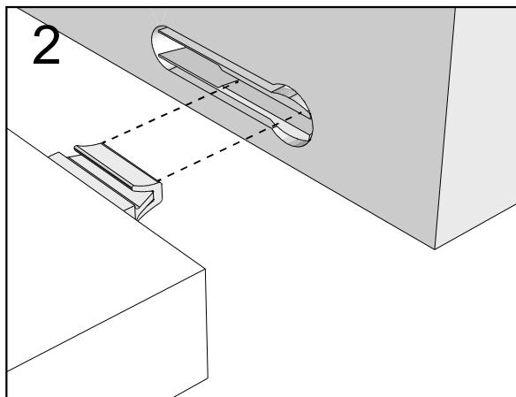
Push connector into housing to join.
