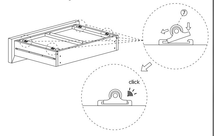
To remove the wheel, push the wheel in and pull it out from the other side as the diagram shows.
