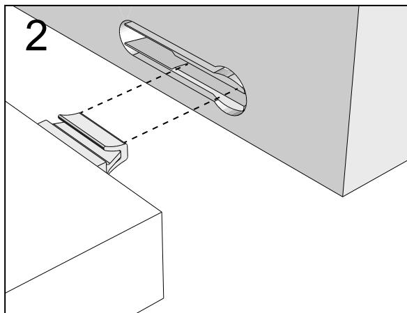
Push connector into housing to be jointed.
