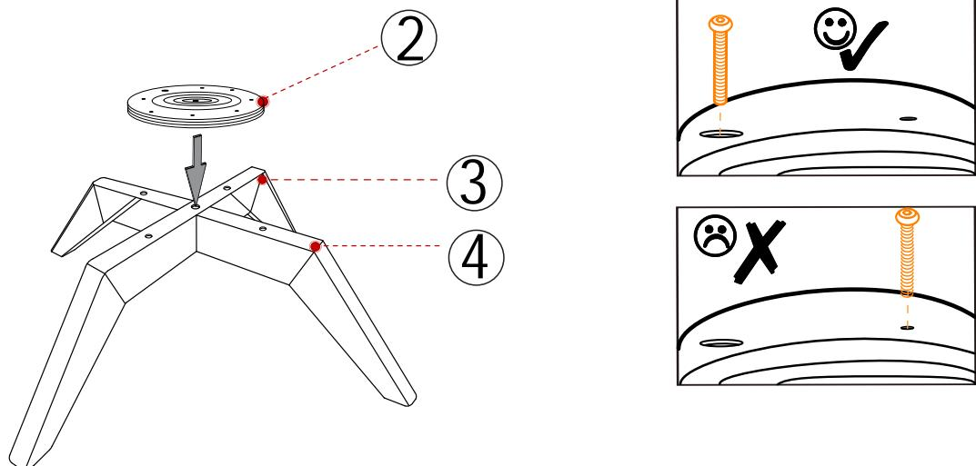
Please rotate the swivel plate, let the big hole align the screw hole, then assembled by the screw, total 4pcs.
