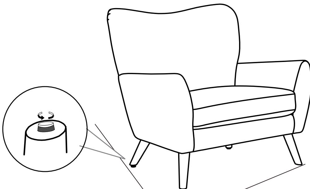
Please adjust the balance of the chair by adjusting the height of the screws.
