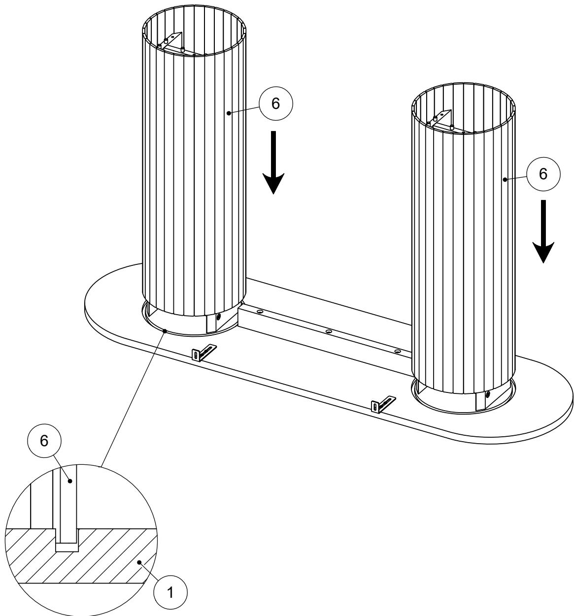
Ensure tambour ribbing is fully inserted within the base.
