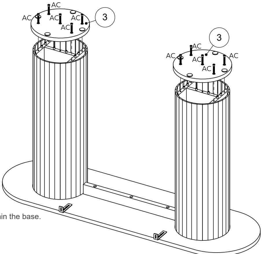
Ensure tambour ribbing is fully inserted within the base.
