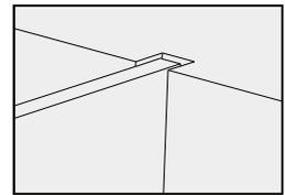
Step2: Press down the two back panels so they are clear of the top panel slot;
