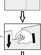
Step2: Press down the two back panels so they are clear of the top panel slot;
