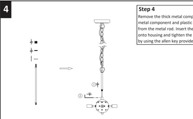
Remove the thick metal component, thin metal component and plastic washer from the metal rod. Insert the metal tube onto housing and tighten the grub screw by using the allen key provided.
