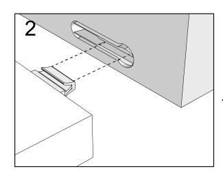
Push connector into housing to join.
