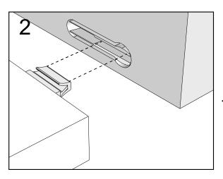
Push connector into housing to join.
