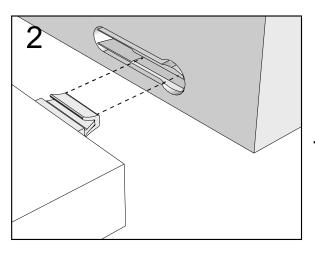
Push connector into housing to join.
