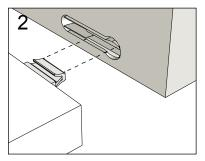
Push connector into housing to be jointed.
