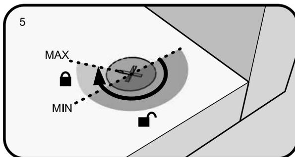
The panels are locked when each cam is turned to between 1/2 and 2/3 of a full turn (Maximum rotation)
