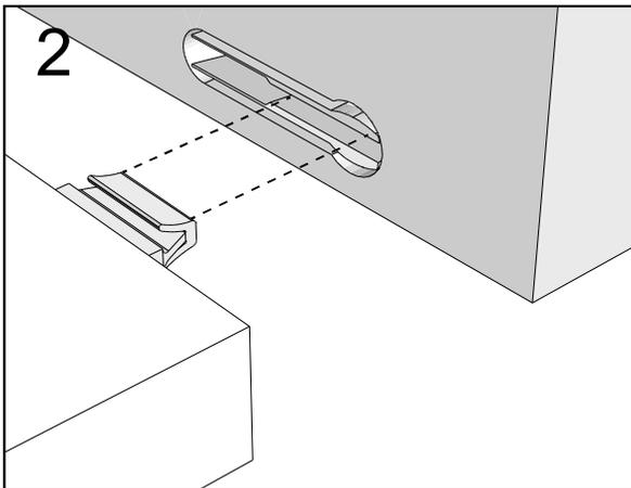
Push connector into housing to join.
