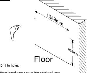
Warning:Always ensure intended wall area to be drilled is free from hidden electrical wires, water and gas pipes.
