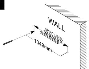
The hole need to be drilled 1049mm apart
