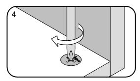
Use a cross-point screwdriver (PH2 or PZ2 is ideal) to tighten the cams and lock the panels together.
