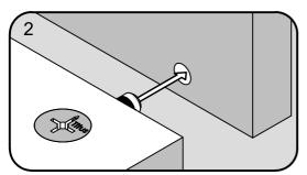
Push the pins into the holes in the panel to be joined.
