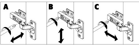
A. Side to side adjustment by clockwise or anticlockwise adjustment .
