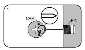
Line up the arrow on the CAM with the PIN.
