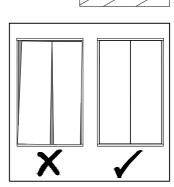
Please ensure all doors and drawers are aligned and evenly spaced before applying the back panel fixings.
