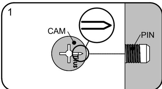
Line up the arrow on the CAM with the PIN.
