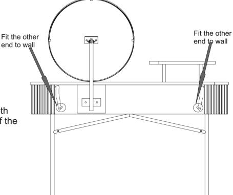
Note: Fit the other end of anti-tip straps provided on both top corners of the rear side of the product to wall
