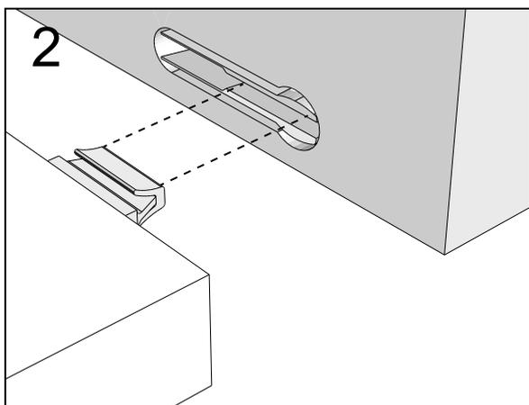
Push connector into housing to be jointed.
