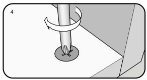
Use a cross-point screwdriver (PH2 or PZ2 is ideal) to tighten the cams and lock the panels together.
