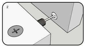
Push the pins into the holes in the panel to be joined.
