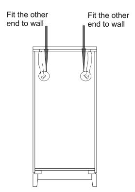
Note: Fit the other end of anti-tip straps provided on both top corners of the rear side of the product to wall
