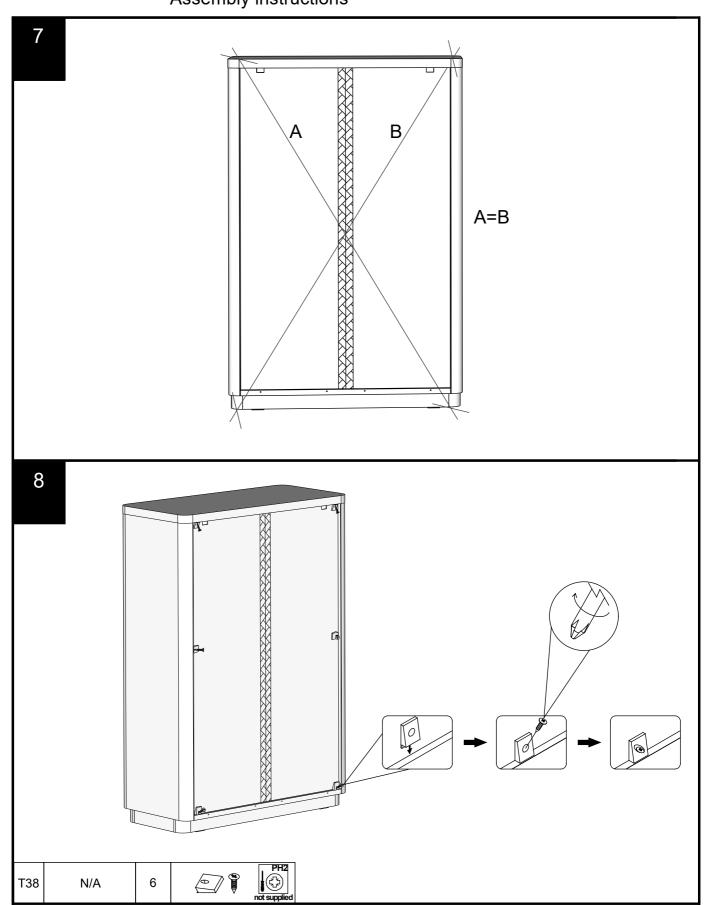
We recommend the use of the wall attachment bracket/strap provided for safety reasons. Move unit into desired position. Secure the 2X"L" metal brackets to the wall with an appropriate screw and wall plug for your wall type (not provided).
