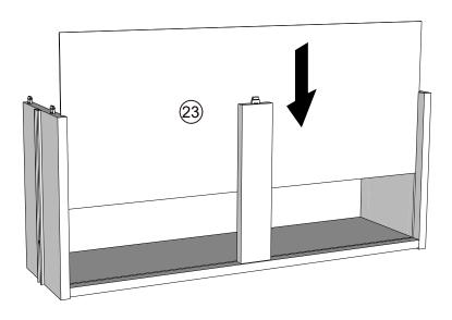
Note: Drawer will be permanently assembled once panel (24) is fitted. ■ 23
