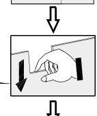
Step2: Press down the two back panels so they are clear of the top panel slot;
