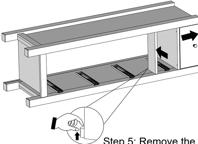
Step 5: Remove the Wood Dowels and Slide the Panel(7) back to unlock
