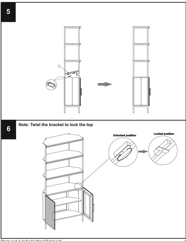
The wall bracket must be fitted for safety reasons.
