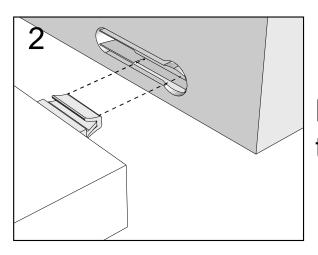
Push connector into housing to join.
