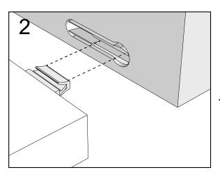
Push connector into housing to join.
