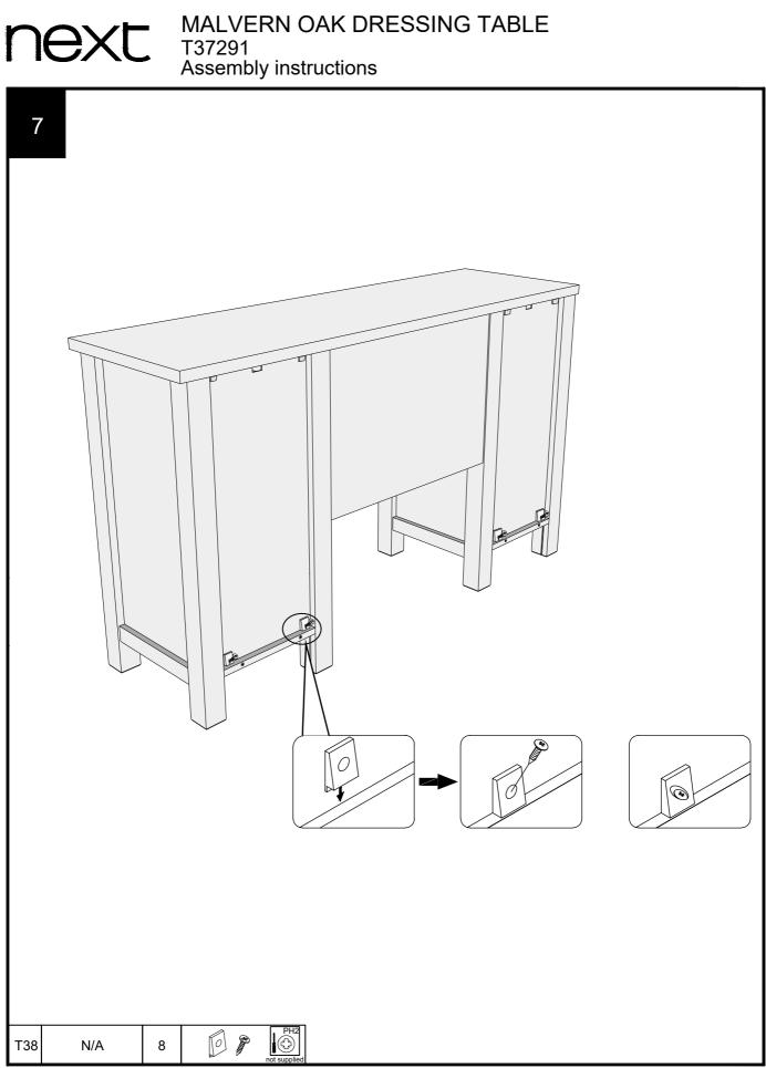
We recommend the use of the wall attachment bracket/strap provided for safety reasons. Secure the strap to the wall with an appropriate screw and wall plug for your wall type (not provided). To hide the strap behind the unit ,drill the hole lower than the top of unit.
