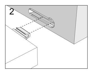
Push connector into housing to be jointed.
