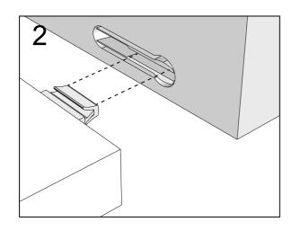
Push connector into housing to be jointed.
