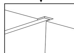
Step2: Press down all the back panels so they are clear of the top panel slot;
