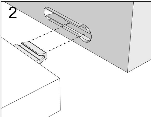
Push connector into housing to be jointed.
