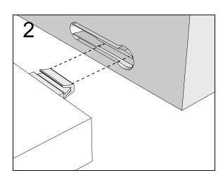
Push connector into housing to be jointed.
