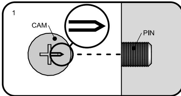
Line up the arrow on the CAM with the PIN.
