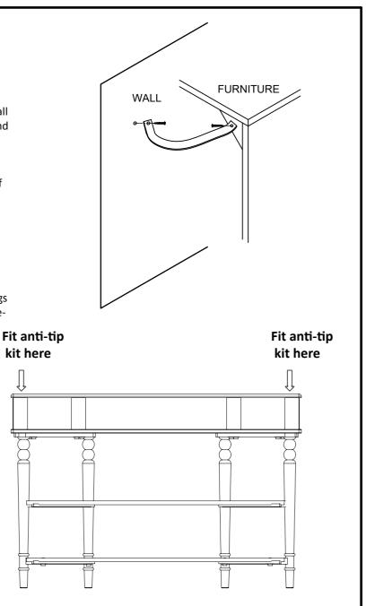
Note: Fit the anti tip straps on both top corners of the rear side of the product and fix the other end of the strap to wall.
