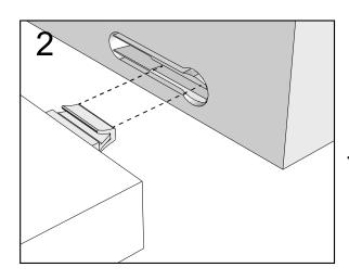
Push connector into housing to be jointed.
