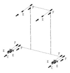
Step 3. Hang the mirror (A) on to the screws and check to ensure that all screws are fully secured. Then insert the shelf (B) into the wall bracket (C) and tighten the grub screws (D).
