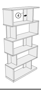
19 Slide the top panel front to unlock, then lift off. Follow the same sequence to remove the other panels.
