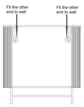
Note: Fit the other end of anti-tip straps provided on both top corners of the rear side of the product to wall
