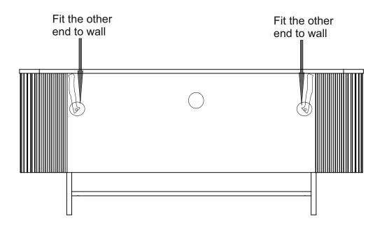
Note: Fit the other end of anti-tip straps provided on both top corners of the rear side of the product to wall
